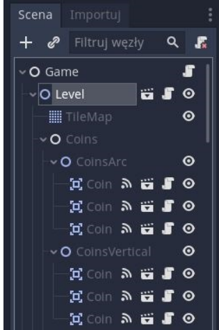
Figure 10: Tree hierarchy of nodes in Godot Engine Figure 11: By moving parent node we move all pinned nodes in Godot Engine
